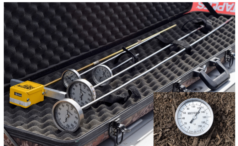
Figure 15. Example of thermometer used to determine the temperature during the pasteurization of field topsoil and other organic materials. Photo by W. Garrett Owen.
