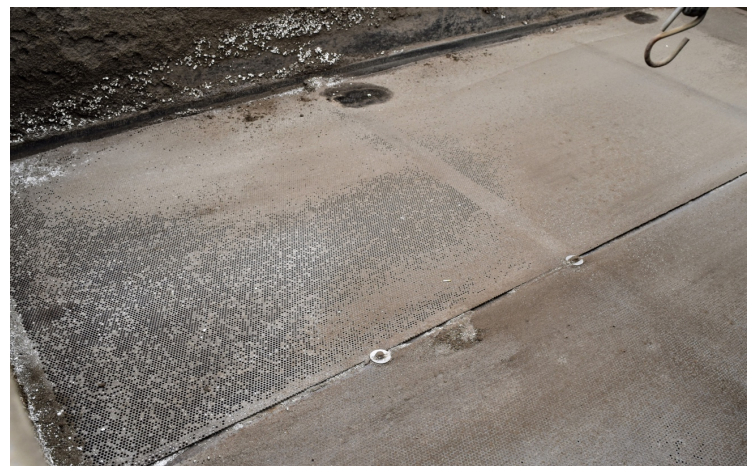
Figure 11. Example of a steam wagon's perforated bottom for field topsoil pasteurization. Photo by W. Garrett Owen.
