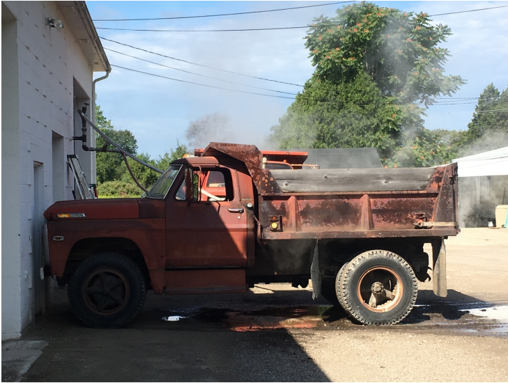
Figure 12. Example of a retro-fitted truck used for field topsoil pasteurization. Photo by W. Garrett Owen.
