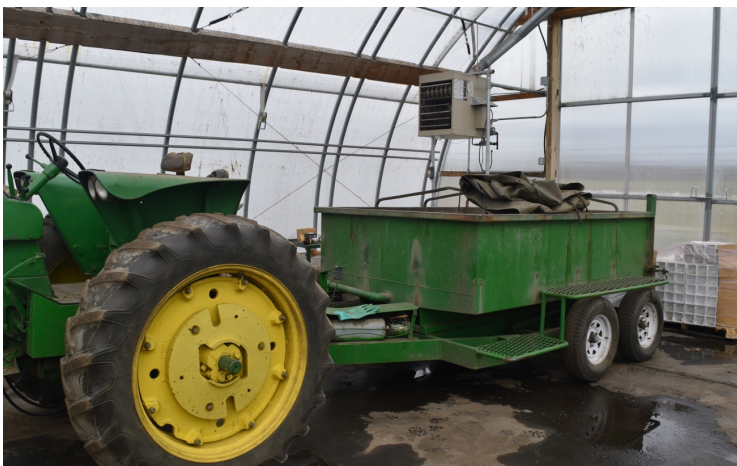
Figure 10. Example of a steam wagon for field topsoil pasteurization. Photo by W. Garrett Owen.
