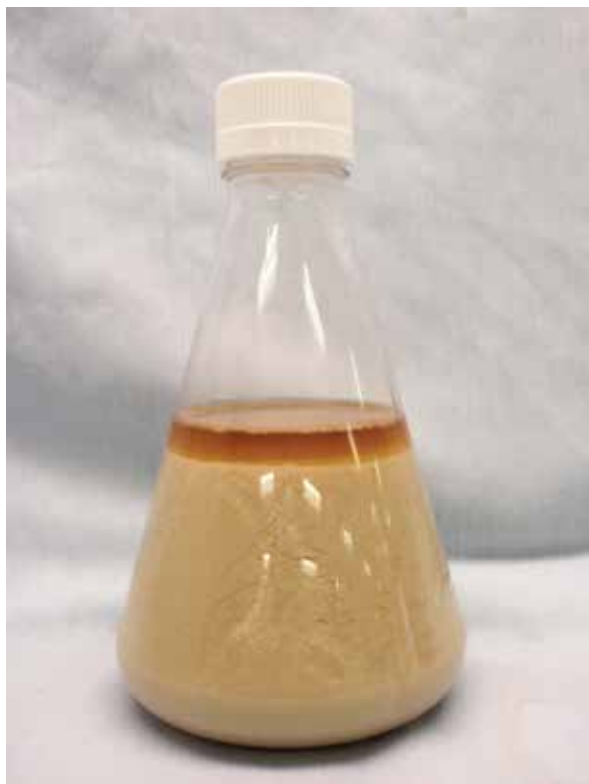
Figure 2. All 0.4% paclobutrazol formulations settle over time. Here, a clear separation of the clay-based particles is seen. The active ingredients settle out within a few days, but aren't visible.
