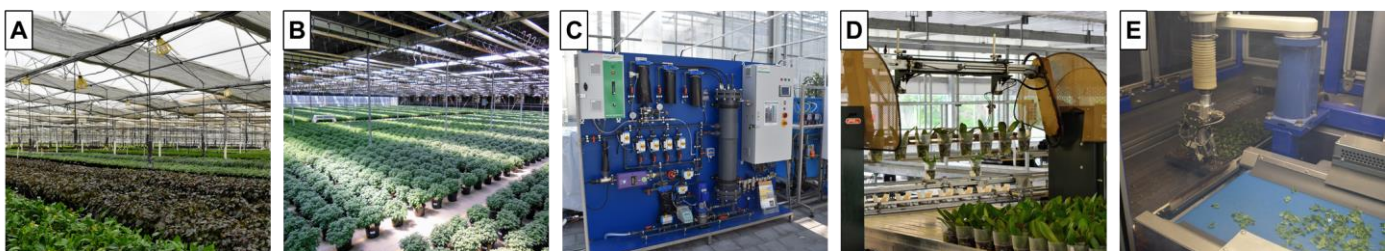
FIGURE 16. Examples of other technologies that may be installed in greenhouses including (A) energy curtains, (B) blackout curtains, (C) advanced water filtration, (D) automation systems, and (E) robots.
